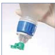
*Bottle with inserted spike ready for aseptic pouring.*
